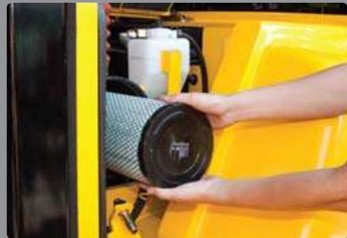
Easy Change Air Cleaner The air filter is readily accessible for cleaning or replacement.
