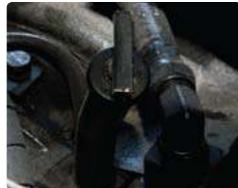
Easy Maintenance Oil Check The T/M oil level can be checked easily without any disassembly.
