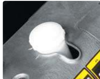
Brake Fluid Reservoir with Level Switch When brake oil level became lower than Min., the warning lamp on the cluster lights on.
